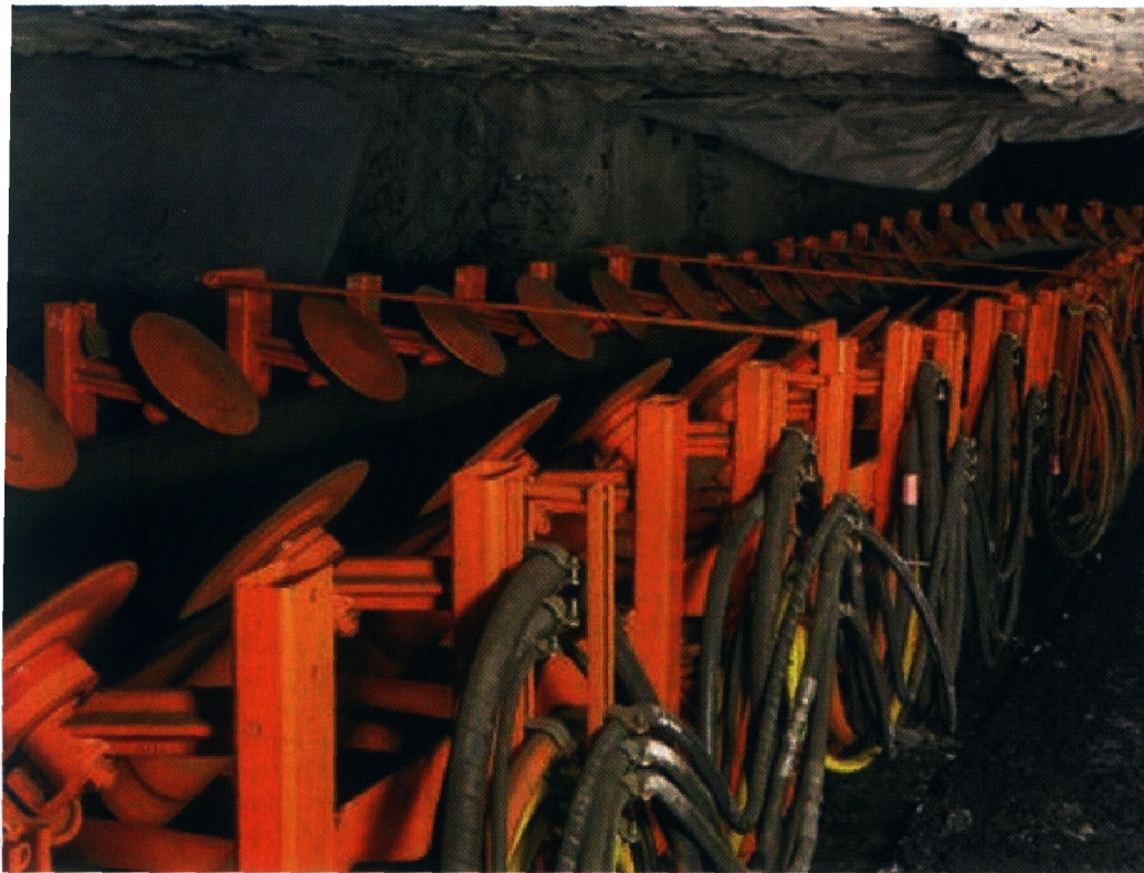
A section of the 4FCT flexible conveyor underground at the Clarence colliery in NSW
